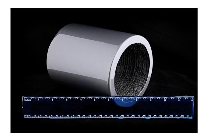
This isotropic, neodymium-iron-boron bonded permanent magnet was 3-Dprinted at DOE's Manufacturing Demonstration Facility at Oak Ridge National Laboratory. Credit: Oak Ridge National Laboratory
