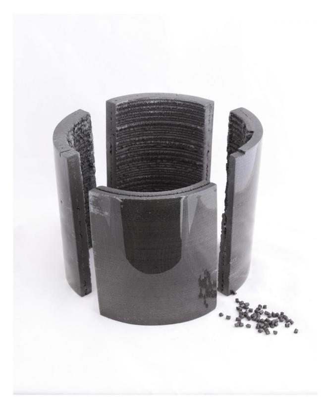
Composite pellets are melted, compounded, and extruded layer-by-layer into desired forms. Credit: Oak Ridge National Laboratory
