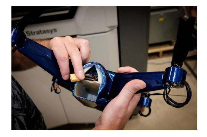
NTU-Stratasys 3D Printed ULTEM drone with embedded electronics. Credit: Nanyang Technological University
