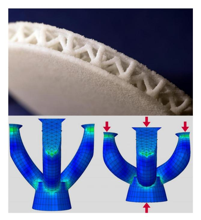
3D structures made of TPU for insoles. These structures were designed using CAD, and their properties were simulated and compared with experiments. Credit: Fraunhofer IWM
