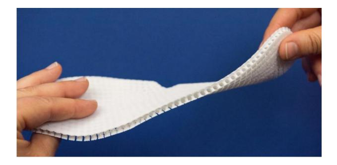
With a combination of different structures in an insole, localized rigidity is digitally adjustable. Credit: Fraunhofer IWM
