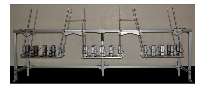
The experimental system consists of three swings connected by springs and holding up to 15 metronomes each. Adjacent metronomes and swings transfer momentum to one another, and adjacent swings transfer momentum through the springs. With the right metronome frequency and spring strength, complex global behavior such as the chimera state can emerge. Credit: Ryan Burrus
