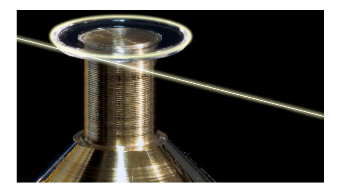
A microresonator crystal used in this study . Credit: © T.J. Kippenberg/EPFL
