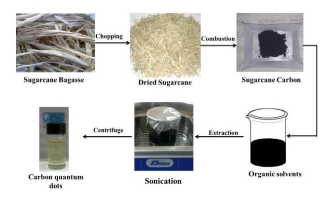
This schematic representation illustrates the process of turning bagasse into carbon quantum dots. Credit: Elsevier
