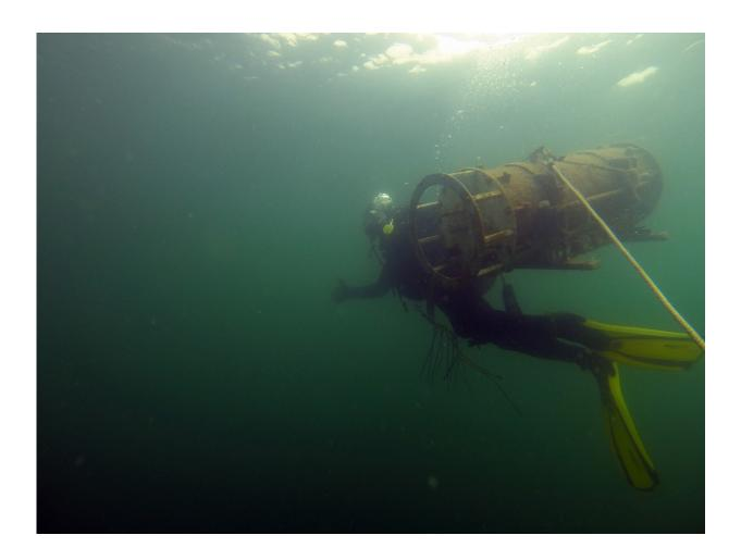
Co-author Alexi Shalapyonok guides FlowCytobot (FCB) to a boat for recovery after being disconnected from the Martha's Vineyard Coastal Observatory. After months of deployment in the ocean, instruments must be recovered for maintenance back at WHOI. Deployment of a second instrument on the same day makes it possible to minimize gaps in the long data records that are critical to uncover multiyear patterns of change in microscopic plankton. Credit: Sean
