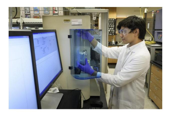
Purdue doctoral student Arthur Dysart operates a system that measures the adsorption of gas molecules on a solid carbon surface. He is working on a team developing materials that capture carbon dioxide, a strategy aimed at reducing the effects of climate change. Credit: Purdue University image/John Underwood
