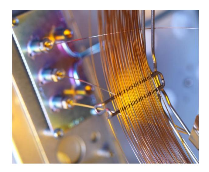
A capillary column used in gas chromatography to separate chemicals. Credit: National Physical Laboratory
