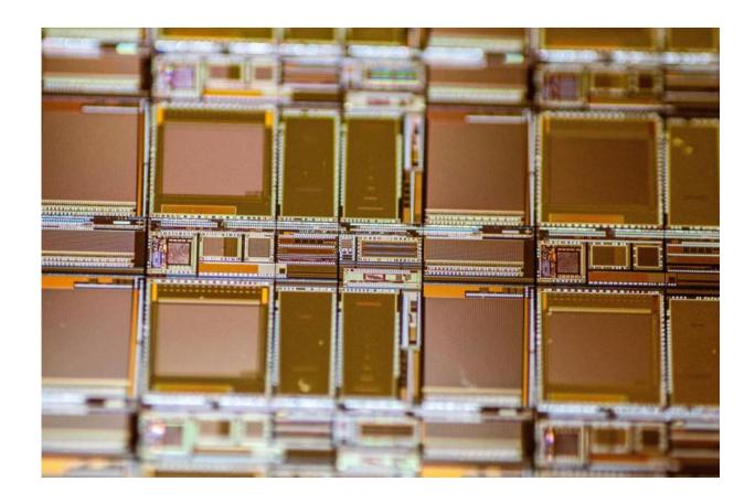
SPAD sensor chips are implemented in CMOS technology. Credit: Fraunhofer IMS
