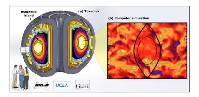
A schematic view of the DIII-D tokamak shows magnetic islands, along side computer simulations of a magnetic island and turbulence. Credit: DIII-D National Fusion Facility
