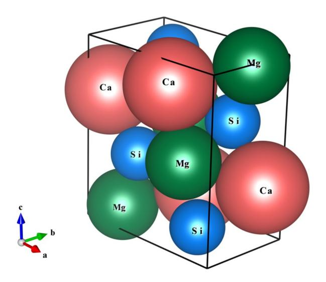
Schematic illustration of the atomic structure of the synthesized CaMgSi determined by X-ray diffraction. Credit: (c) Toyohashi University Of Technology.
