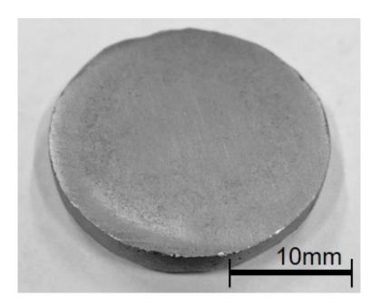
Picture of the synthesized bulk CaMgSi thermoelectric material through the procedure developed in this study. Credit: (c) Toyohashi University Of Technology.
