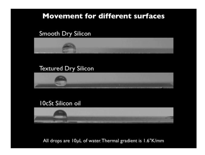
This animation shows the response of droplets on silicon surfaces, showing that untreated or textured surfaces do not allow the droplets to move in response to temperature differences, but that on a surface with a lubricant on a textured surface, the droplets move easily. Video has been sped up. Credit: Henri-Louis Girard/Varanasi Research Group
