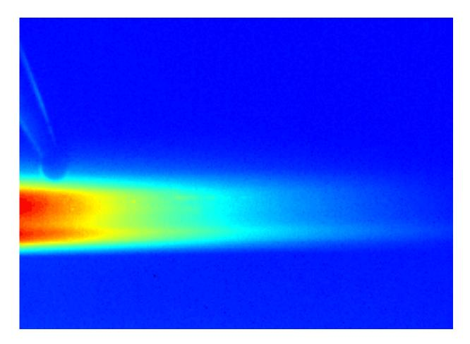
This animation is an infrared side view of the motion of a droplet as it moves across a treated silicon surface in response to temperature differences on that surface. It demonstrates how the droplet initially equilibrates in temperature with the substrate and then, as it moves, continues to be in thermal equilibrium with the surface. Credit: N. Bjelobrk/Varanasi Research Group
