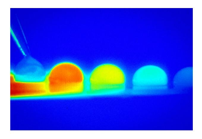
In a time-lapse sequence, infrared imaging shows the temperature changes within a droplet of water as it moves across a treated silicon surface in response to temperature differences on that surface. Credit: N. Bjelobrk/Varanasi Research Group. Edited by MIT News
