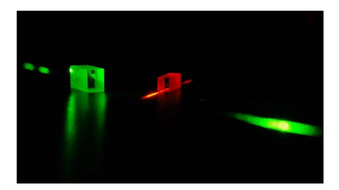
This image shows crystals used for storing entangled photons, which behave as
