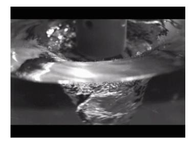
Rotary Jet-Spinning (RJS) works likes a cotton candy machine. A liquid polymer solution is loaded into a reservoir and pushed out through a tiny opening by centrifugal force as the device spins. As the solution leaves the reservoir, the solvent evaporates and the polymers solidify and elongate into small, thin fibers. Credit: Harvard University
