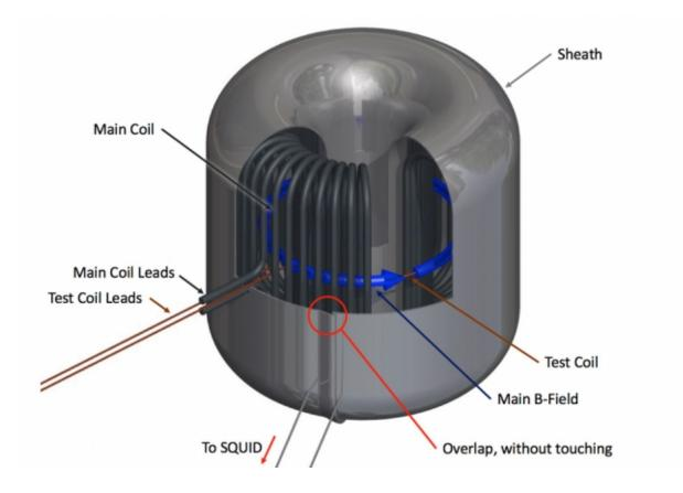
A sketch of the ABRACADABRA toroidal magnet. A constant magnetic field circulating around the toroid can interact with axion dark matter to produce a small oscillating magnetic flux through the center. In the absence of axion dark matter, this flux would be zero. Credit: Daniel Winklehner
