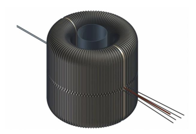
ABRACADABRA (A Broadband/Resonant Approach to Cosmic Axion Detection with an Amplifying B-field Ring Apparatus), consists of a series of magnetic coils, wound in the shape of a toroid, or donut, which is then encased in a layer of superconducting metal and kept at temperatures just above absolute zero. The scientists plan to use a highly sensitive magnetometer, placed inside the donut hole, to detect any signs of axions' influence. Credit: Daniel Winklehner
