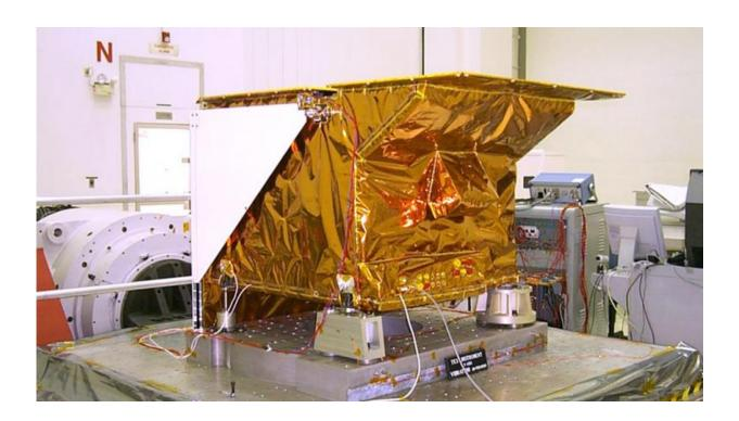
NASA's Tropospheric Emission Spectrometer (TES) instrument, one of four instruments on NASA's Aura spacecraft. Credit: Northrop Grumman
