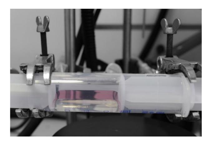
Formation of a stable layer of chemically bonded gold nanoparticles with the smallest possible thickness -- that is, a monolayer (visible in purple). Image taken in the laboratory of the Institute of Physical Chemistry of the Polish Academy of Sciences in Warsaw Credit: IPC PAS, Grzegorz Krzyzewski
