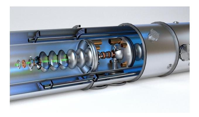
The SNS LINAC is the most powerful proton-pulsed accelerator in the world. Stretching the length of nearly three football fields, the LINAC is responsible for focusing and propelling protons to roughly 90 percent the speed of light just before they smash into a liquid mercury target, releasing about 25 neutrons for every proton to be used for scientific discovery. Credit: ORNL/Jill Hemman, et. al.
