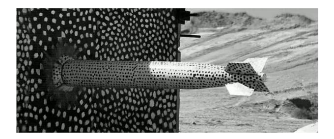
A B61-12 test unit slams into a target at the end of Sandia National Laboratories' 10,000-foot rocket sled track in a complex forward ballistics test. The test, which mimicked a high-speed accident, allowed engineers to examine safety features inside the weapon. Credit: Sandia National Laboratories
