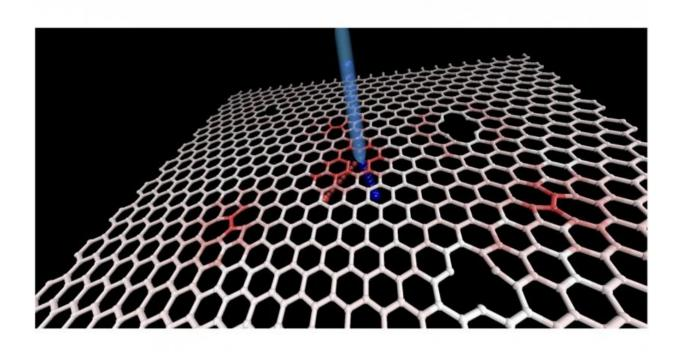
A simulation shows the path for the collision of a krypton ion (blue) with a defected graphene sheet and subsequent formation of a carbon vacancy (red). Red shades indicate local strain in the graphene. Credit: Kichul Yoon, Penn State
