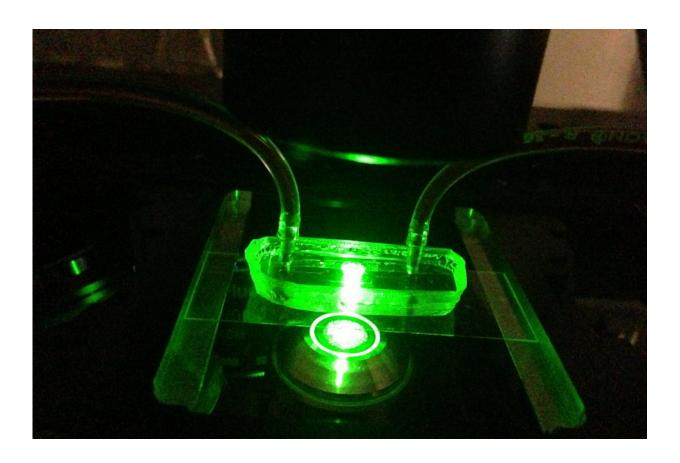
University of Connecticut researchers used a fluorescence microscope to illuminate a microfluidic device that simulates a blood vessel. The research team was able to observe and measure how particles of different sizes behave in the bloodstream. Their finding, that particle size matters, could aid the development of more effective cancer drugs. Credit: Anson Ma/University of Connecticut
