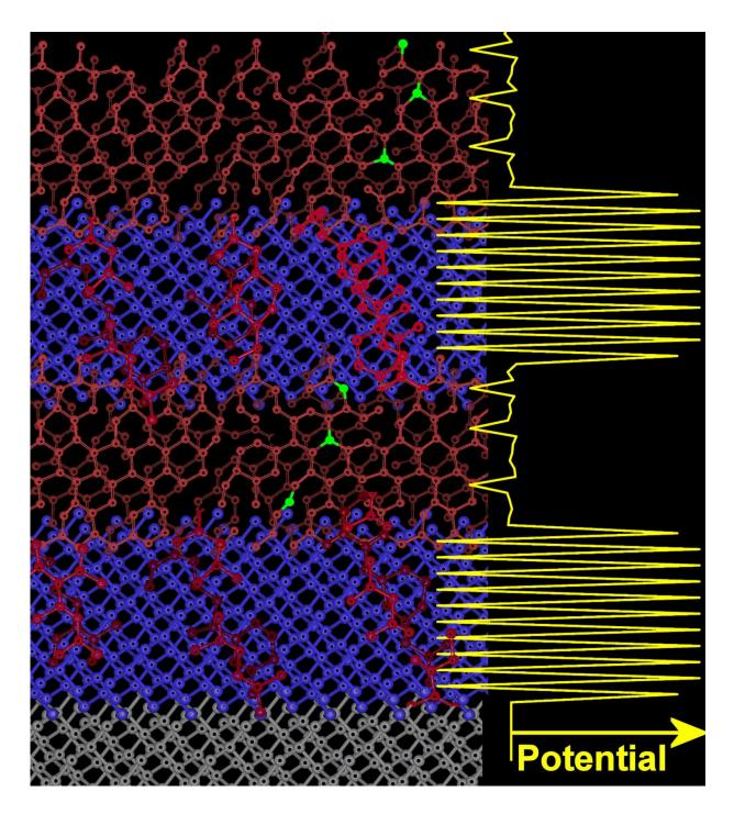
A schematic atomic diagram of a quantum well made from amorphous carbon layers. The blue atoms represent amorphous carbon with a high percentage of diamond-like carbon. The maroon atoms represent amorphous carbon which is graphite-like. The diamond-like regions have a high potential (diamond is insulating) while the graphite-like regions are more metallic. This creates a quantum well as electrons are confined within the graphite-like region due to the
