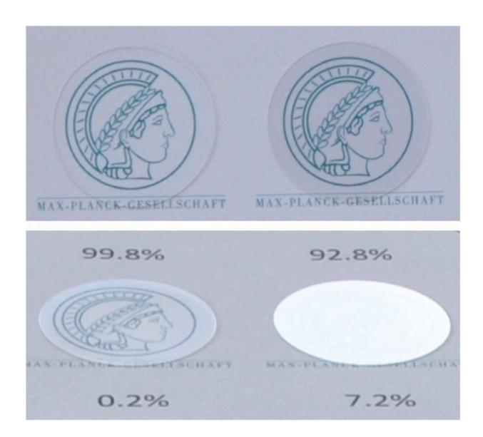
Image of the Greek goddess Minerva as seen under a fused silica substrate with 450 nm nanopillars on both sides (left) compared to an unstructured reference
