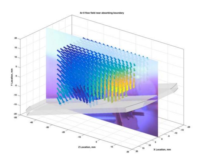
Measured flow field of ions in a plasma overlaid on visual image of the system. Credit: West Virginia University
