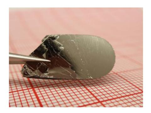
A crystal sample of one of the iron-based unconventional superconductorsstudied by Ames Laboratory scientists. Their systematic investigation of this class of superconductors may lead to the creation of new materials with unique superconducting properties. Credit: U.S. Department of Energy, Ames Laboratory
