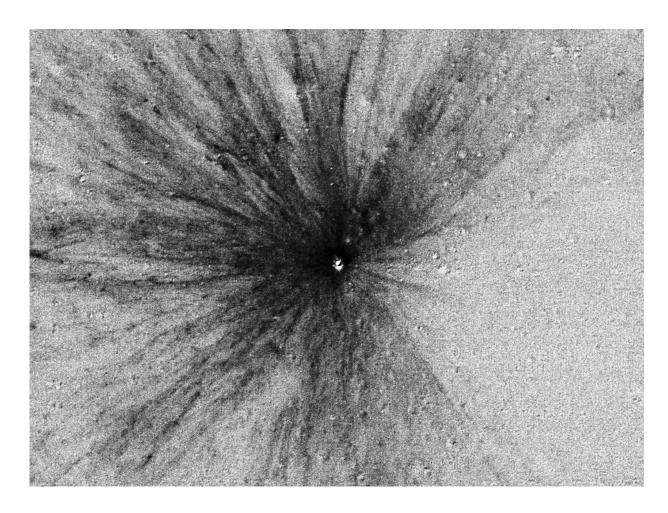
To reveal the pattern of debris from the 12-meter crater impact, the team divided the "after" image by the "before" image. The result brings out a striking starburst pattern — and shows that some debris flew farther than 150 crater-diameters. The image is 1,300 meters (4,300 feet) wide. Credit: NASA/GSFC/Arizona State University
