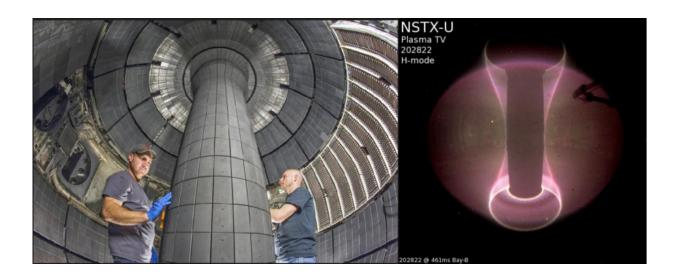
The new NSTX-U center stack central magnet that doubles the magnetic field and plasma current, left, and an image of NSTX-U H-mode plasma. Credit: Elle Starkman/PPPL Office of Communications. Right: NSTX-U Team.
