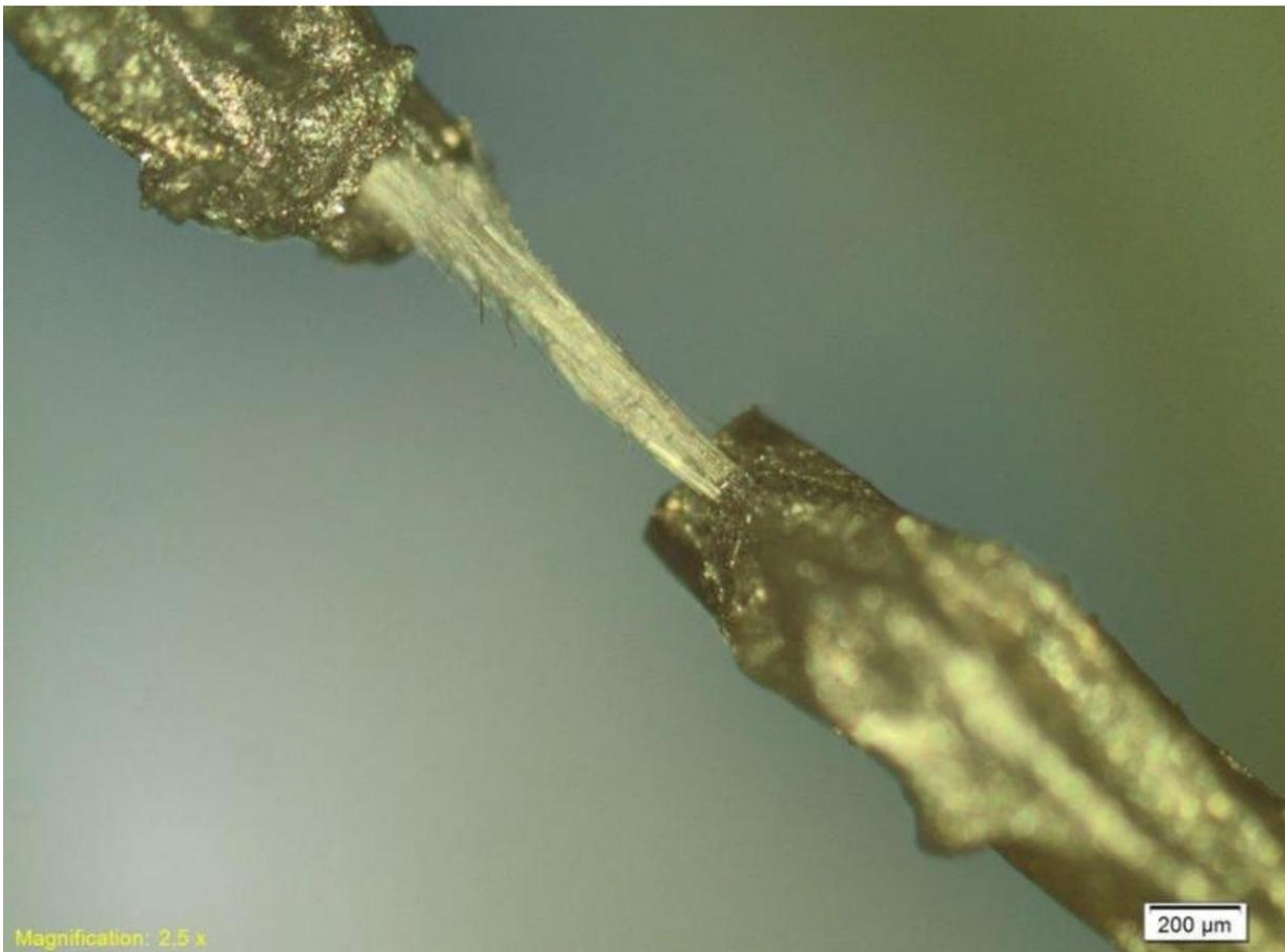
An optical image of the microtube bundle placed between two electrodes. Credit: Kholkin et al., Applied Physics Letters
