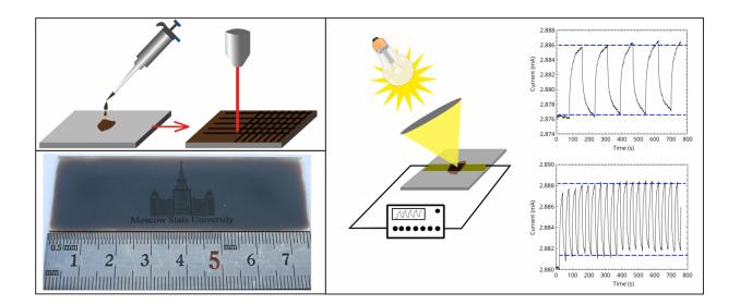
A schematic of the structuring of graphene oxide: Photo microstructuring; Prototype circuit of the bolometer and its work. Credit: Stanislav Evlashin
