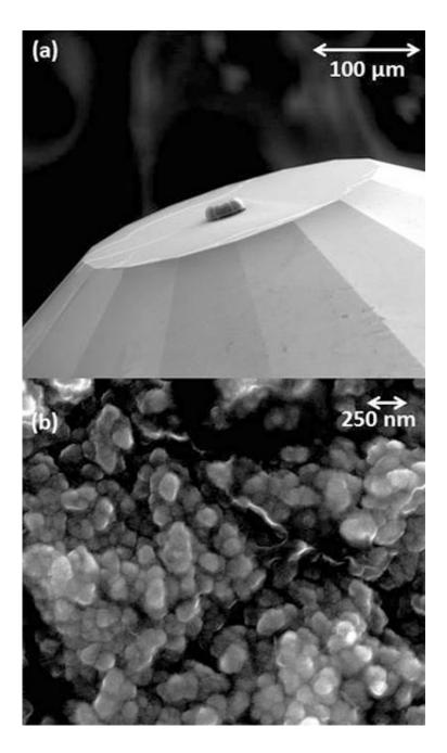
This nubbin on the flat surface of a gem diamond (top) is a nanocrystalline diamond, half the width of an average human hair. Higher magnification (bottom) shows the granular structure of the nanocrystalline diamond. Credit: University of Alabama at Birmingham
