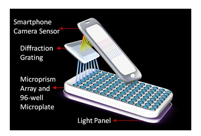
Washington State University researchers have developed a low-cost, portable laboratory on a smartphone that can analyze several samples at once to catch a cancer biomarker, producing lab quality results. Credit: Washington State University
