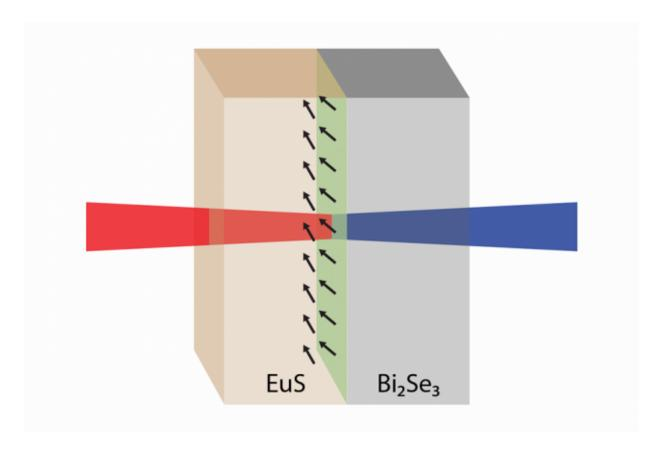
Figure 1: An external magnet orients the internal magnetism of a sandwiched europium sulfide and bismuth selenide film in one direction. A phenomenon called magnetic second harmonic generation changes a small fraction of red laser light passing through this magnetic field into blue light, which can be measured to reveal the direction and strength of magnetism between the layers. Credit: Changmin Lee
