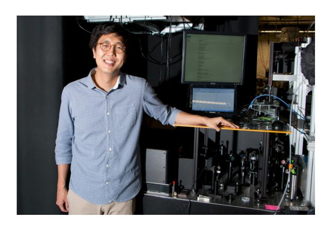
MIT graduate student Changmin Lee stands by an experimental setup that uses light pulses to map the magnetic direction and strength of a buried interface between two exotic materials, bismuth selenide and europium sulfide. Credit: Denis Paiste/Materials Processing Center
