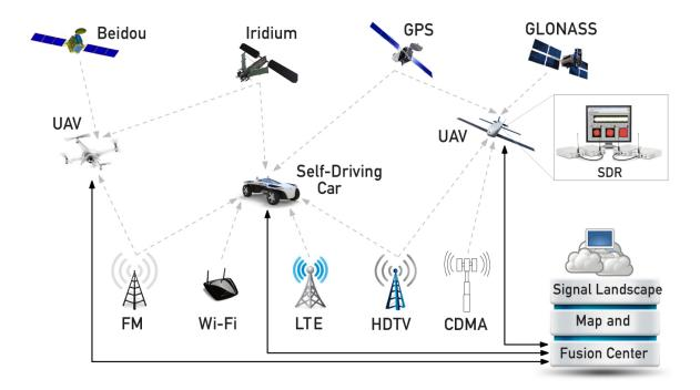
A schematic showing how researchers at UC Riverside are using existing communications signals to complement satellite-based navigation systems like GPS for the control of driverless cars and unmanned aerial vehicles (UAVs). Credit: University of California - Riverside
