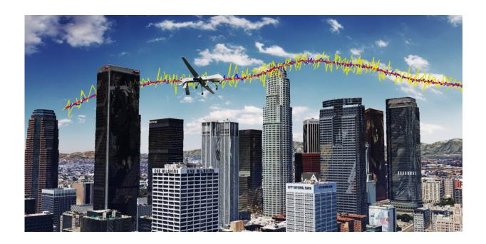
Simulation results for an unmanned drone flying over downtown Los Angeles showing the true trajectory (red line), with GPS navigation only (yellow line), and GPS aided with cellular signals (blue line). Credit: University of California - Riverside
