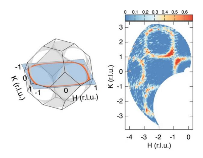
Left: A "spiral surface" (grey) as predicted by theoretical studies. The red ring shows a cut within a two-dimensional plane in reciprocal space. Right: Diffuse scattering intensities observed in the same plane at low temperatures. Credit: Copyright: S. Gao + O. Zaharko (Paul Scherrer Institut, Switzerland)
