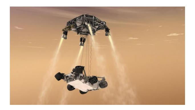
NASA's Mars 2020 rover will use a landing system nearly identical to the 2012 landing of Curiosity (depicted in this artist's concept) but with added precision from the Lander Vision System. Credit: NASA/JPL-Caltech
