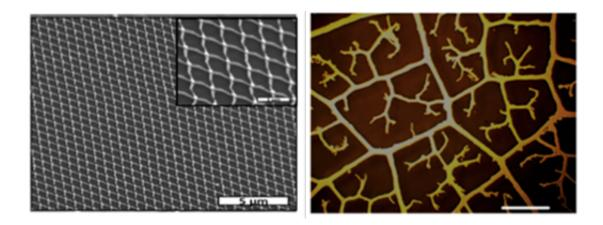
SEM -- model of a metallic nano-network with periodic arrangement (left) and visual representation of a fractal pattern (right). Credit: HZB/M. Giersig
