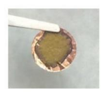
Graphite/PMMA/Li trilayer electrode before (left) and after (right) being soaked in battery electrolyte for 24 hours. Before soaking in electrolyte, the trilayer electrode is stable in air. After soaking, lithium reacts with graphite and the color turns golden. Credit: Yuan Yang, Columbia Engineering
