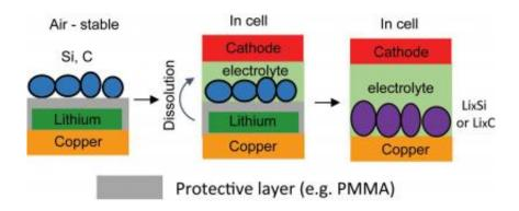
Illustration showing the procedure to fabricate the trilayer electrode. PMMA is used to protect lithium and make the trilayer electrode stable in ambient air. PMMA is dissolved in battery electrolyte and graphite contacts with lithium to compensate the loss due to reduction of electrolyte. Credit: Yuan Yang, Columbia Engineering
