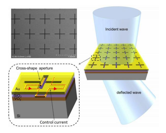
Figure showing how the metamaterial, with cross-chaped openings, can deflect a terahertz beam's angle. Credit: University of California, Los Angeles
