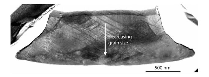
A cross-section composite image of a silver microcube impacted on its side shows decreasing grain size closer to where the deformed cube hit the target. Rice University scientists believe their research will lead to better materials for high-impact applications. Credit: Thomas Group/Rice University
