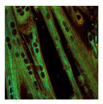
Fluorescence lifetime imaged on a color scale — at higher temperatures, the fluorescent dye loses its fluorescence more rapidly, which can be detected to measure temperature change. Credit: Royal Society of Chemistry
