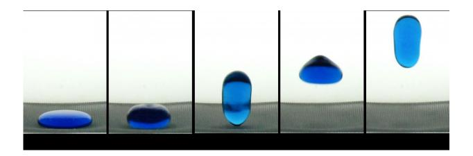
A 2-mL "puddle" of water spontaneously jumps from a hydrophobic surface upon release into a freefall. Credit: Weislogel
