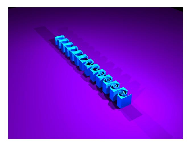
A computer rendering if the 12 different kinds of spirals contained in the metamaterial blocks, each of which slows sound waves by a specific amount. Organizing the various spirals in an array can bend the shape of in incoming wave of sound. Credit: Steve Cummer, Duke University
