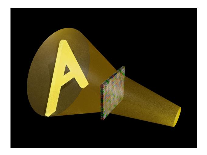
A computer rendering of a sound wave that traveled through an array of acoustic metamaterial and was shaped into a pattern like the letter A one foot past the array. This pattern could not be seen, only heard. Credit: Steve Cummer, Duke University
