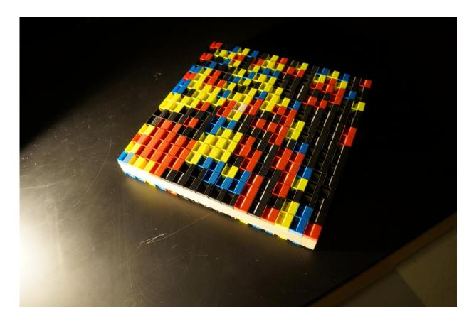
A close up look at the metamaterial device that can create acoustic holograms. Each grid or block contains a spiral of one of 12 various densities, each of which slows sound waves by a different amount. Credit: Steve Cummer, Duke University
