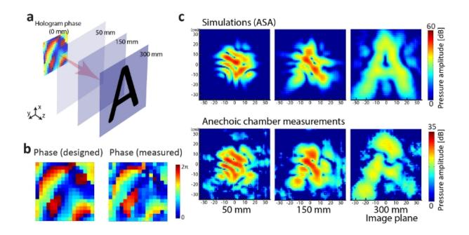
Computer simulations and experimental results of the effectiveness of the metamaterial acoustic hologram device producing the letter A. The sound wave was manipulated to create the letter A 300mm past the metamaterial device. Test results show a result close to calculations. Credit: Duke University
