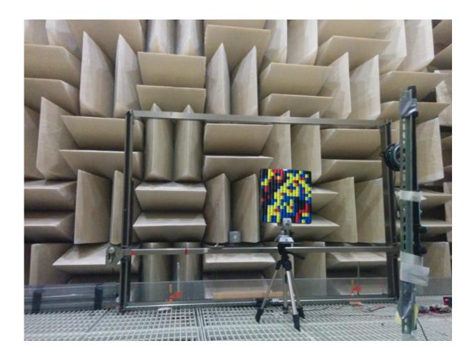
The metamaterial device is set up for testing in front of a sound-absorbing wall so that reflecting sound waves do not affect the experiments. Credit: Duke University
