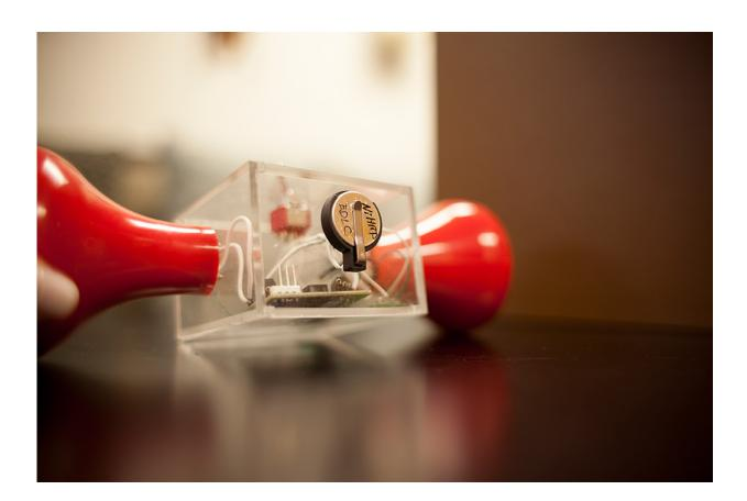
To demonstrate the supercapacitor's ability to store power, the researchers modified an off-the-shelf hand-crank flashlight (the red parts at each side) by cutting it in half and installing a small supercapacitor in the center, in a conventional button battery case, seen at top. When the crank is turned to provide power to the flashlight, the light continues to glow long after the cranking stops, thanks to the stored energy. Credit: Melanie Gonick
