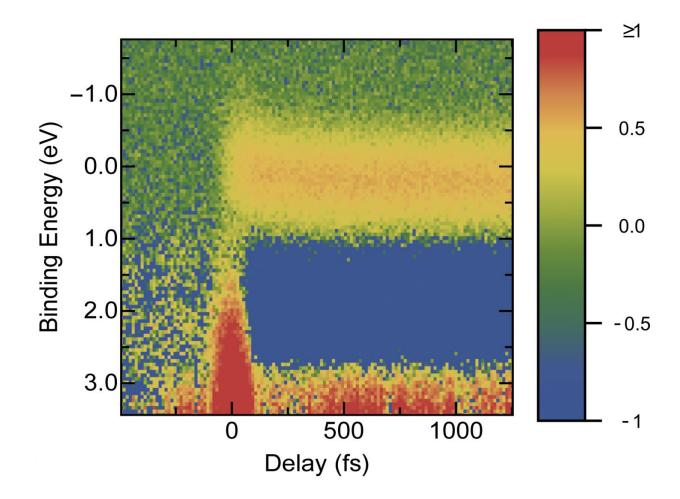
This graph shows the relative amount of electrons (coloured scale, right) at a given binding energy shortly after the pump pulse. This information helps to reconstruct how electrons relax from their excited states to the ground state. Credit: HZB
