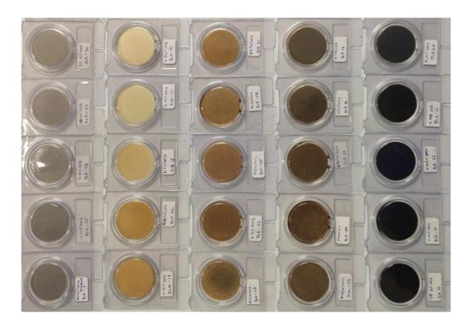
A set of test filters used to collect organic compounds in smoke from roadside trash fires in India were turned a rainbow of toxic colors, rather than the usual shades of gray one would expect from ambient air filtering. "One of my labmates thought I was looking at a panel of eye shadows," said researcher Heidi
