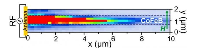
Figure 1 – 2D distribution of spin-waves propagation in a 1µm wide CoFeB conduit recorded using Brillouin light scattering spectroscopy (BLS).
