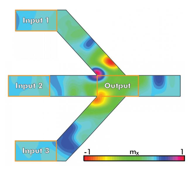
Figure 2 – Fork structure of a majority gate consisting of input and output magneto-electric cells integrated in a spin-wave bus. The picture shows a snapshot at t=0.8ns when inputs are 110. Credit: imec
