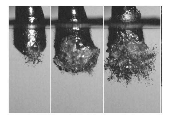
Vapor explosion of an 8 mm diameter drop of liquid Field's metal as it falls into a pool of water. Credit: KAUST
