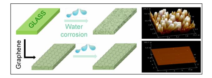
Graphene coatings protect glass from corrosion as shown in the atomic force microscopy images on the right. On uncoated glass (top right), the surface roughness increases after immersion in water for 120 days. In contrast, glass plates coated with graphene films were much more stable and the increase in roughness was negligible after immersion in water for 120 days. Credit: Reprinted with permission from Bin Wang et al, ACS Nano 2016. Copyright 2016 American Chemical Society
