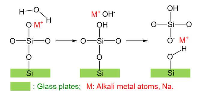
Corrosion mechanism on the glass surface. Credit: Reprinted with permission from Bin Wang et al, ACS Nano 2016. Copyright 2016 American Chemical Society
