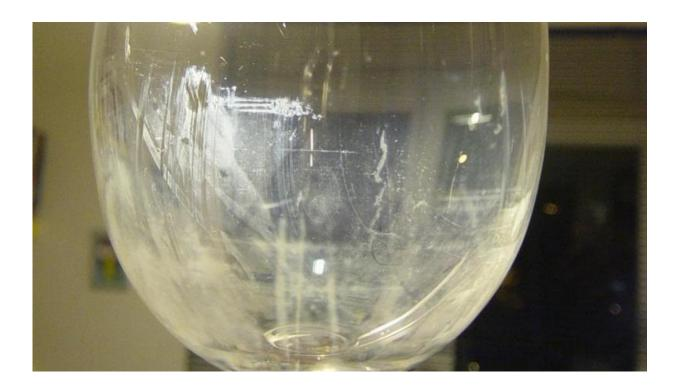
An example of a glass showing cracking and opacity due to corrosion. Credit: Wikipedia
