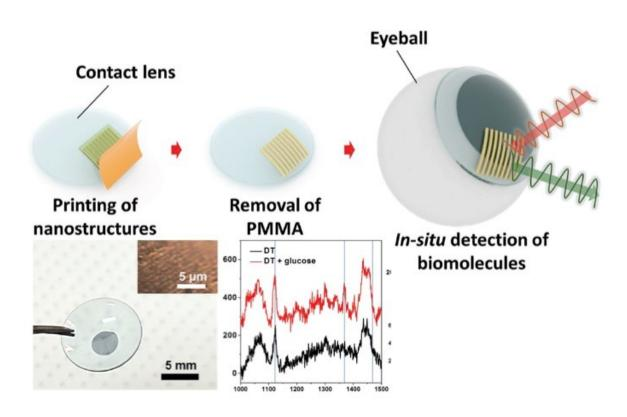
Schematic procedure for the fabrication of a surface-enhanced Raman scattering contact lens via transfer printing. Credit: University of Houston
